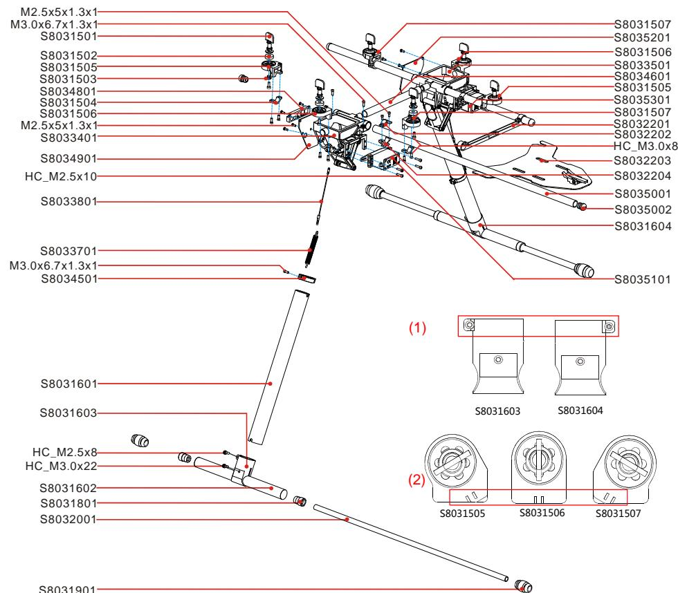
Note: (1) Left and right T-Frame are different; (2) Left set, middle set and right set of carbon tube bracket are different.
