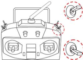
**Retracted** :Toggle the switch to this position to retract the landing gear (Fig.1)
