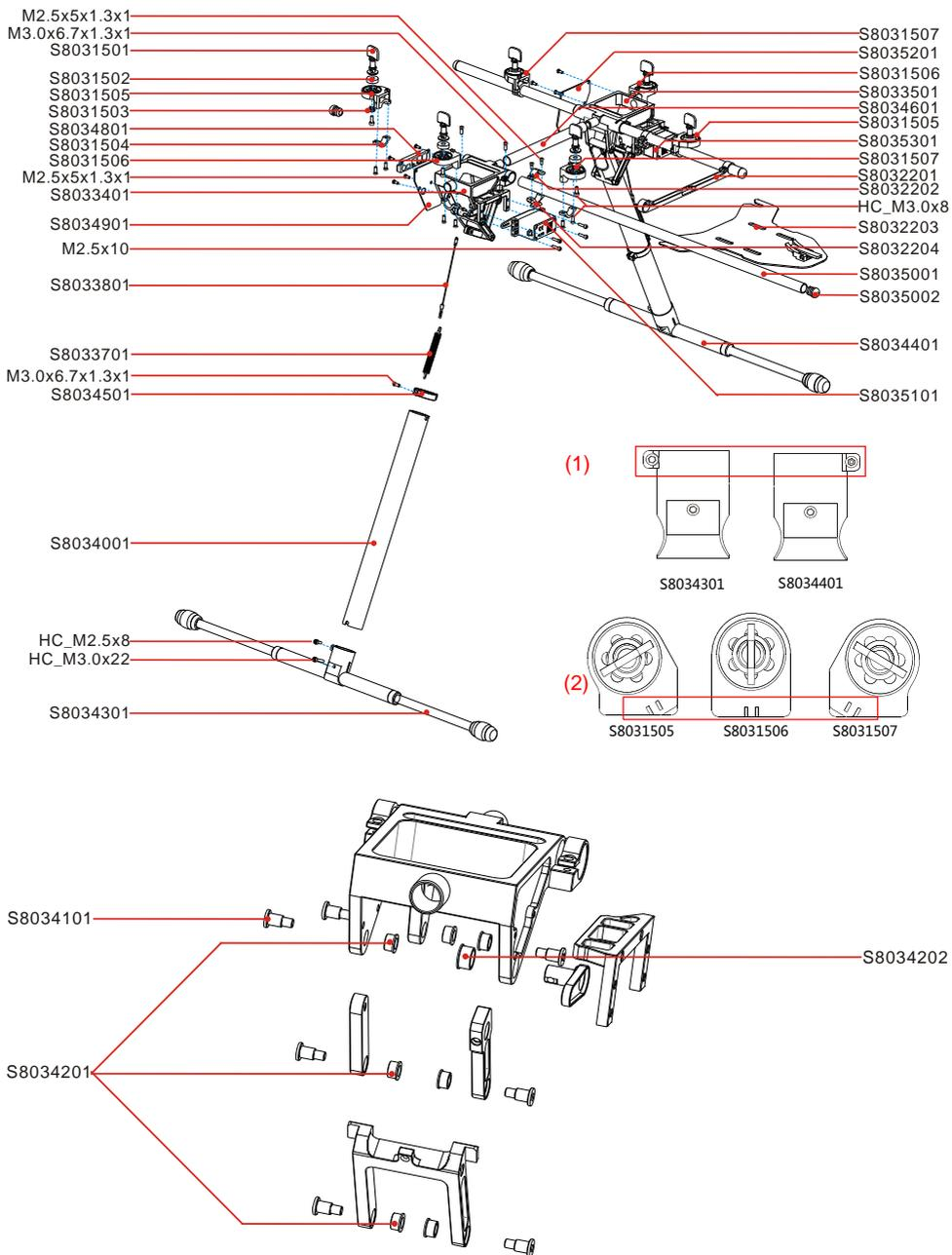
Note: (1) Left and right Bottom Frame are different; (2) Left set, middle set and right set of carbon tube bracket are different.
