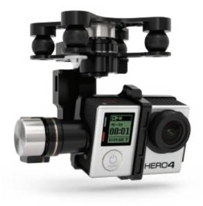
Fly your **GoPro Hero4 Black** camera with this custom-built gimbal. The **DJI Zenmuse H4-3D** was designed specifically for this camera, and perfectly stabilizes it in the air while allowing tilt control when used with a compatible flight platform.
